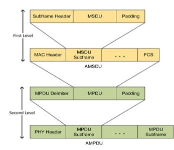
Fig. 7. Two level of frame aggregation.
