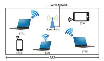
Fig. 3. A typical 802.11 wireless infrastructure network with five STAs.
