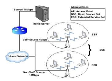
Fig. 14. VoIP over WLAN Industrial Integration Architecture System.
