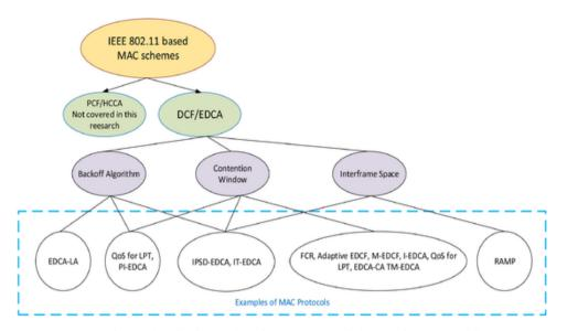
Fig. 12. Approaches used in the design of wireless MAC protocols for providing service differentiation.
