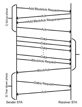
Fig. 8. IEEE 8902.11 (EDCA) BlockAck Mechanism.
