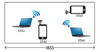
Fig. 4. A typical 802.11 wireless ad-hoc network with four STAs.
