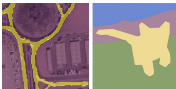
Figure 2.15: Example of semantic segmentation (pixel classification) in deep learning (Esri, 2021d).
