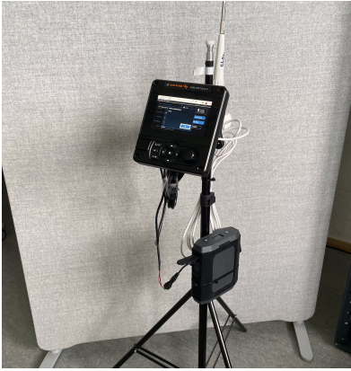
Figure 4.3: The A200 connected to a battery and a VHF antenna
