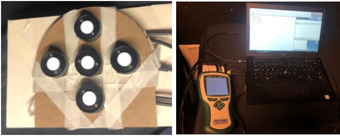
Figure 8. (left) Measurement instrument using Almemo Ahlborn, with photosensors fixed on a circular plate and placed at the tube's exit; (right) logging of measured data via Almemo logger and Almemo control 6.0 software.
