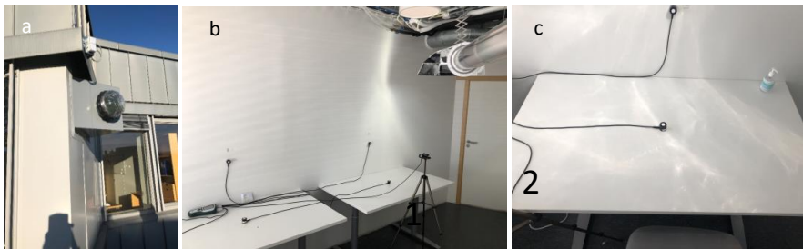
Fig. 5. Light pipe mounted on the facade in the room and an adaptation element for angled mounting (5a); two working areas in the room (5b); light patches on the 2nd desk delivered from the HLP and via the custom-made reflector (5c)
