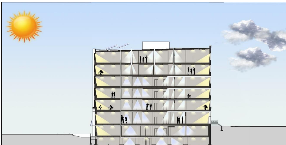
Figure 4 Integrated solution for daylighting (with daylight transport systems [DTS]) and artificial lighting, adopted from (Gentile, Osterhaus et al. 2021) 4 . https://www.iea-shc.org/ All rights reserved.
