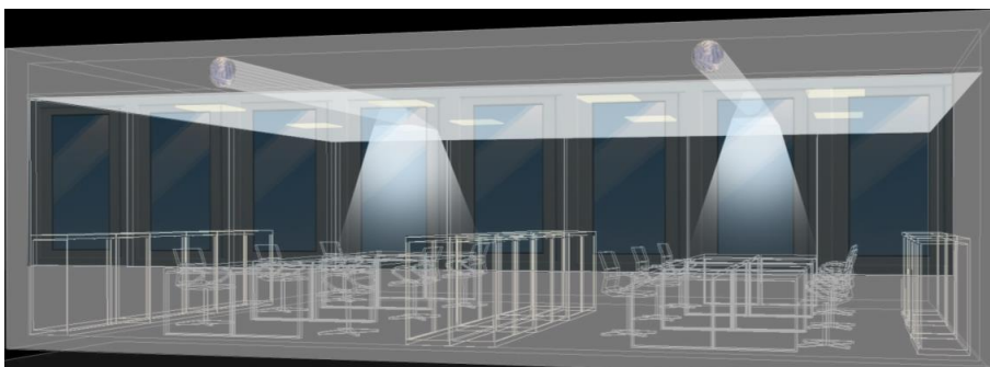
Figure 61 Illustration of HLP applicability in an open plan office space for daylighting of areas far from the windows
