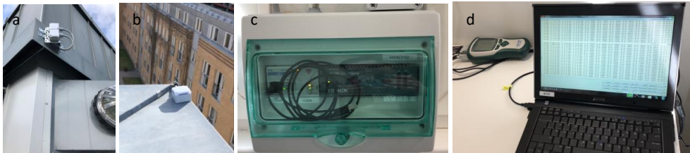
Fig. 7. Monitoring equipment: a) Monitoring of the VI incident to the HLP, VI im; b) monitoring of the GHI, GHI im; c) logging of energy consumption of each luminaire; d) logging of the indoor illuminance measurements from the five photosensors Pim1-5.
