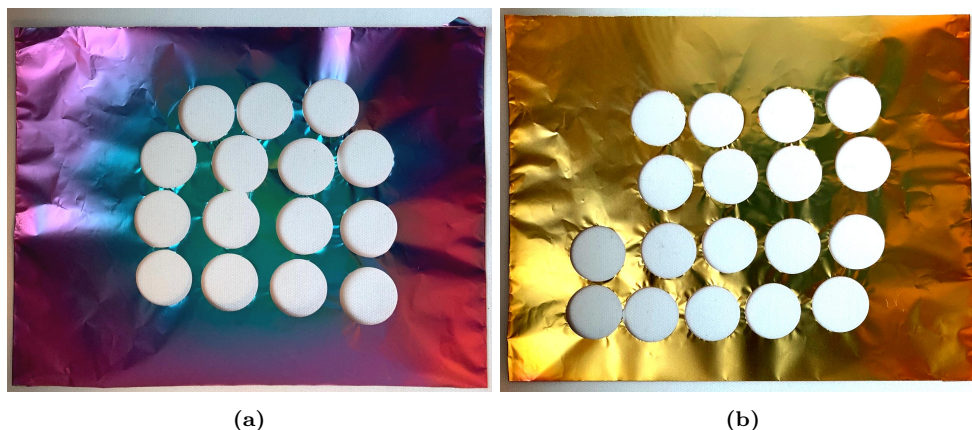
Fig. 5.1.1: The original thin film sheets. The circular holes are where the 15 mm discs used in the coin cells were punched out from. a) Pure Si film. b) \text{SiC}_x film.
