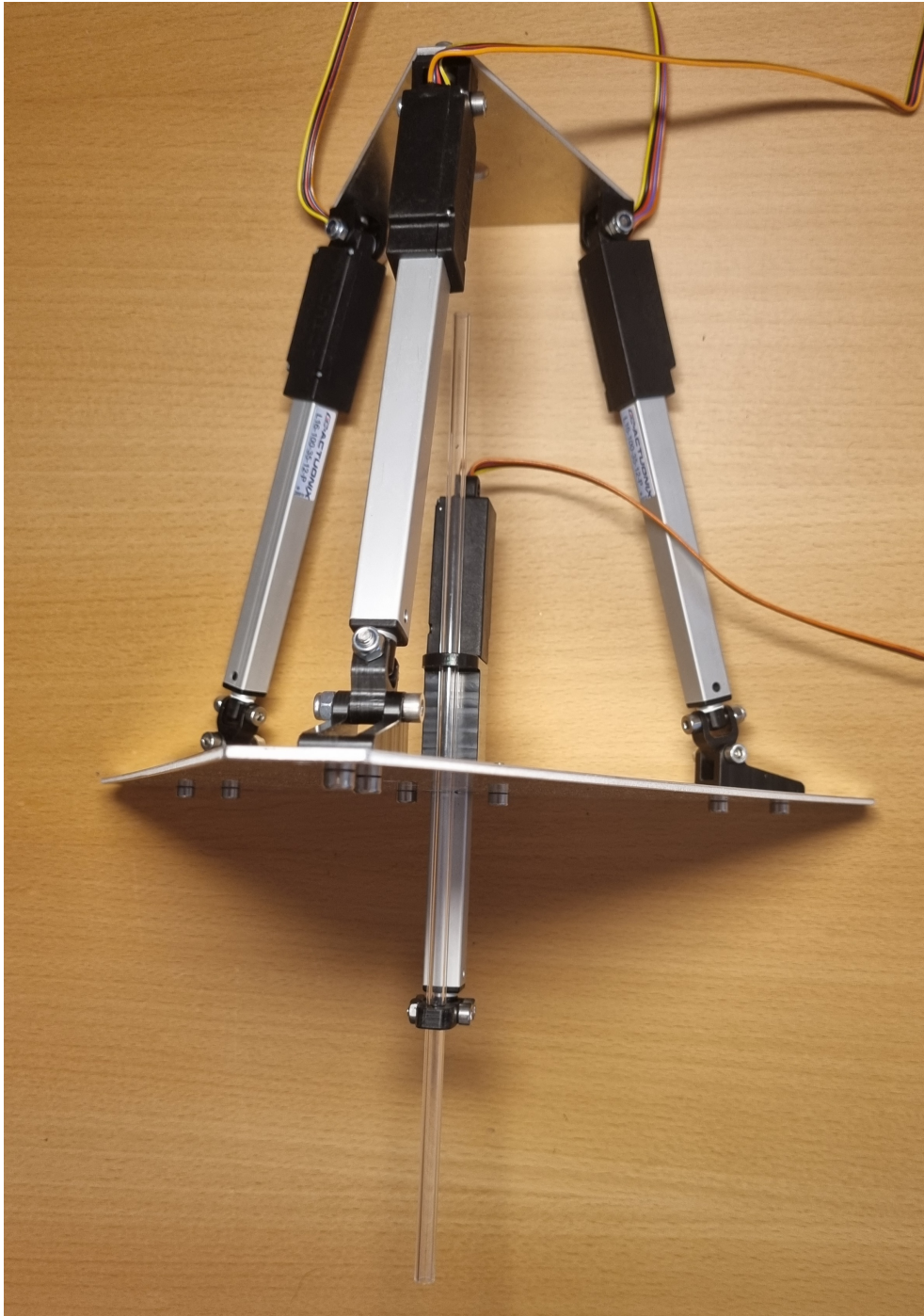
Figure 3.4: The Stewart Platform-Inspired Mechanism
