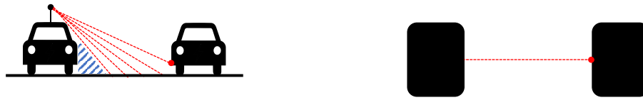
Figure 7.7.: Creation of a Circogram ray from several LiDAR rays. The red lines to the left illustrates laser rays, and the striped blue area close to the car with the LiDAR illustrates a deadspot that the LiDAR cannot detect. The upper red line in the image to the left hits the other car. The image to the right shows the resulting Circogram ray from above the cars.
