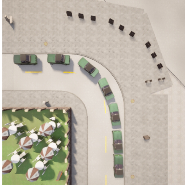
Figure 11.2.: The first driving situation in the testing route. This shows the result of a left turn when navigation command is to follow lane. Seven snapshots of the ego vehicle are stitched together to this figure.
