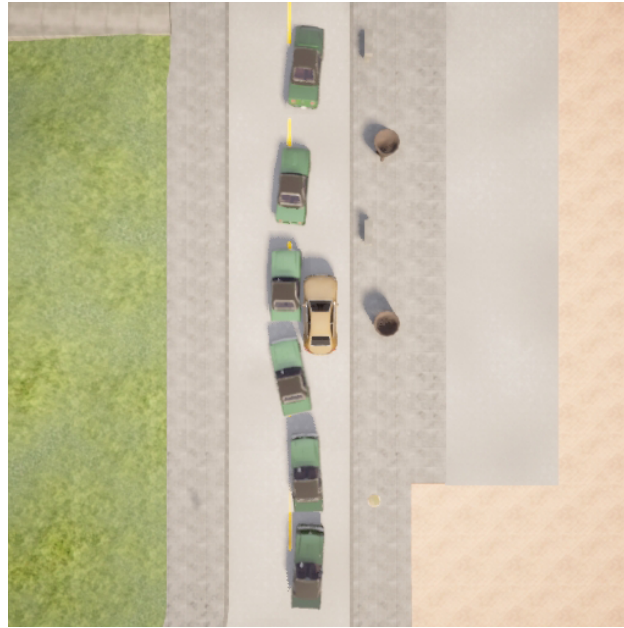
Figure 11.8.: The result of overtaking a parked car in the middle of the lane. Six snapshots of the ego vehicle are stitched together to this figure.
