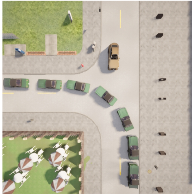
Figure 11.3.: The second driving situation in the testing route. This shows the result of left at intersection with static car. Seven snapshots of the ego vehicle are stitched together to this figure.
