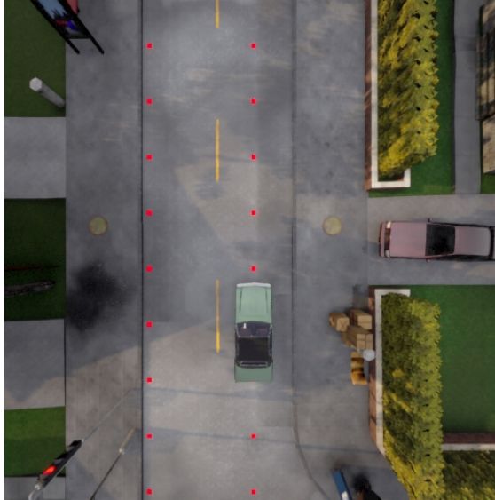
Figure B.1.: Points that are used to create the affine transformation between the coordinate frames.
