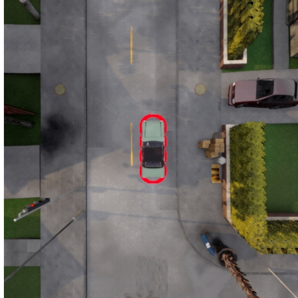
Figure 9.11.: Illustration of four circles that approximate the outer surface of the ego vehicle.
