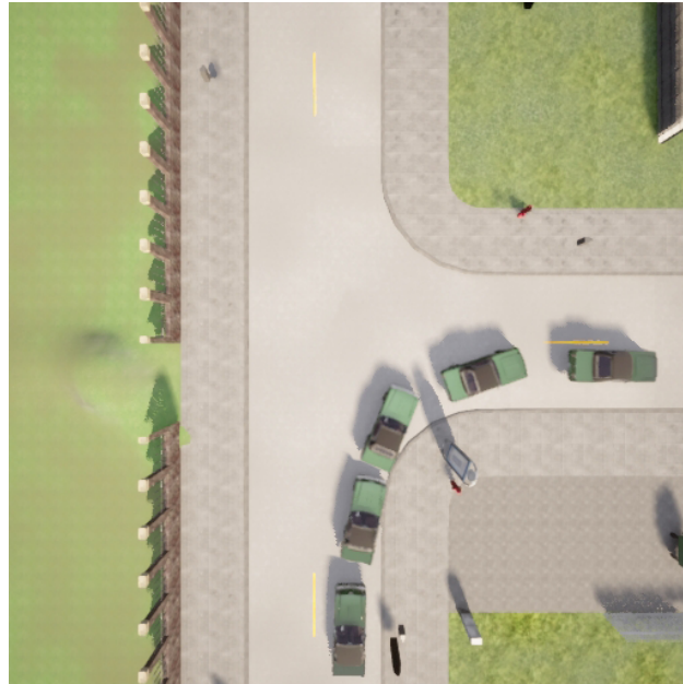
Figure 11.4.: The result of right at intersection without other vehicles. This driving situation contains the sharpest curve the ego vehicle need to drive. Five snapshots of the ego vehicle are stitched together to this figure.
