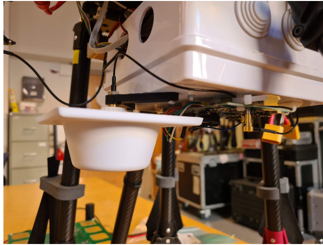
Figure 4.19: RHCP antenna mounted on the multirotor UAV, pointing downwards.
