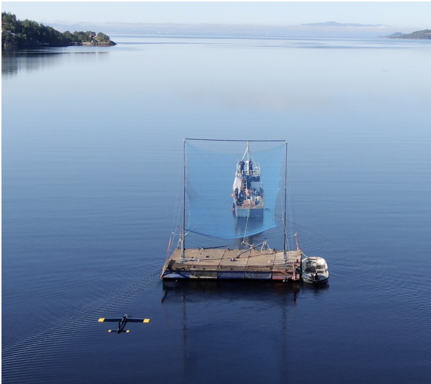
Figure 7.14: UAV approaching the barge-mounted net towed by the ship
