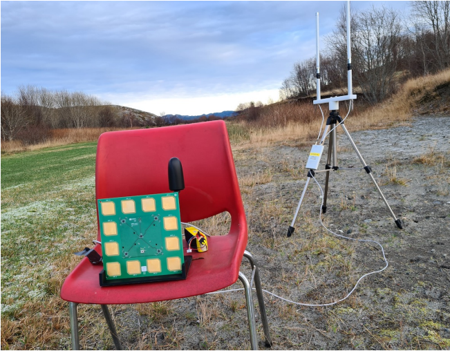
Figure 4.22: Array setup with Ubiquiti Rocket radio for remote equipment placement.
