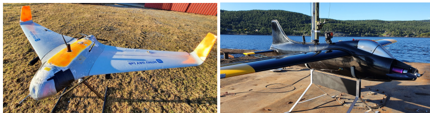
(a) The NTNU Skywalker X8 flying wing (b) The Maritime Robotics Dolphine UAV UAV
