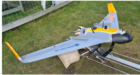
Figure 8.17: Skywalker X8 UAV. The GNSS antenna used for the RTK GNSS rover receiver is the cylinder-shaped component on top of the fuselage. The Bluetooth transmitter antenna is hidden inside the UAV behind the black canvas tape.
