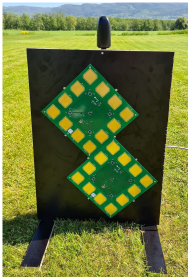
Figure 5.23: Array setup. Data from the lower array was used in the outdoor experiment. Element 11 as per Fig. 5.1 is highest above ground, and element 5 is the lowest.
