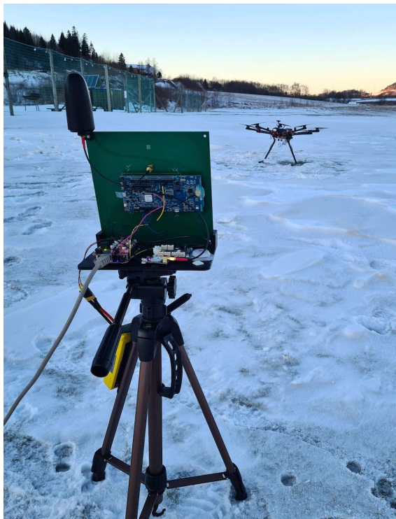
Figure 4.31: The antenna array on a tripod, with array center height 0.7 m over the ground. The DJI S1000 UAV is visible in the background.
