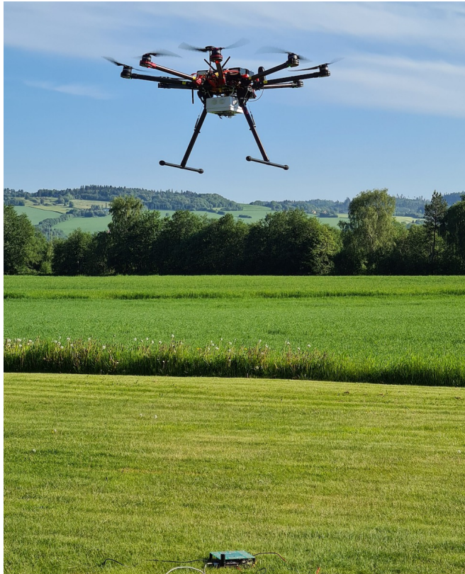
Figure 4.16: Multirotor UAV flying above the array, which is placed flat on the ground facing upwards. The PCB trace antenna on the transmitter board was used.
