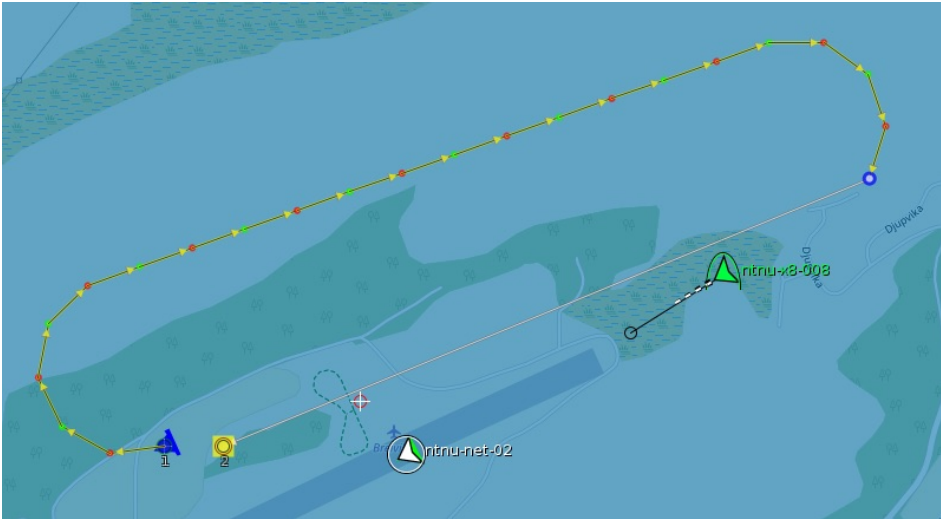
Figure 7.8: The recovery plan generation GUI, with the start position (blue), the arrest system (white), the UAV (green) and the plan inbetween. The small black circle ahead of the UAV corresponds to the carrot point, while the dynamic plan is not in the map view.
