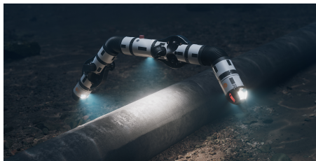
d Underwater inspection and intervention robot performing dual side pipe inspection. Courtesy of Eelume.
