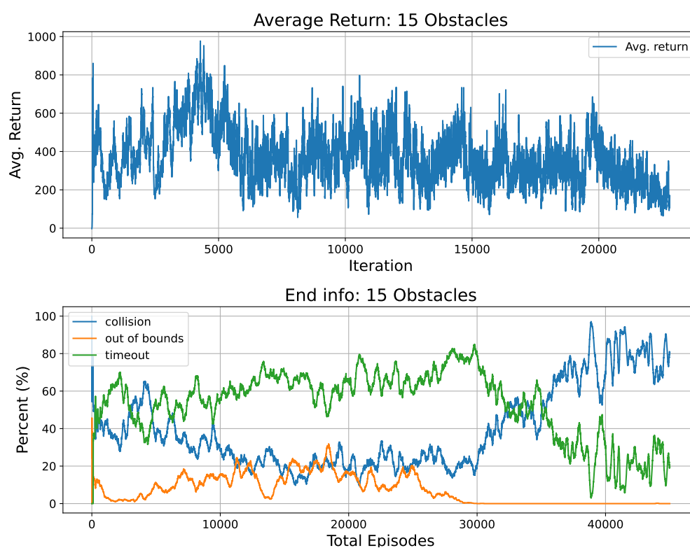
Figure C.1: Training the navigation policy with 15 obstacles in an environments of size [24, 12]. The best model is selected at 4410 iterations.
