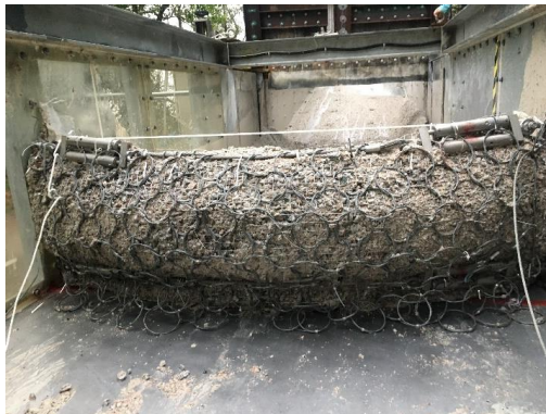
Flexible barrier after a flume test
