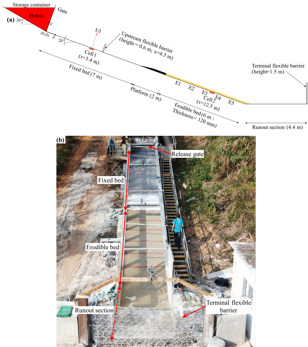
Fig. 3 Flume model: (a) cross-section with instrumentation layout (U refers to ultrasonic sensor; E refers to the erosion column; Cell 1 measures flow basal normal and shear stresses; and Cell 2 measures
