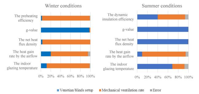
Fig. 3. The overall thermal and fluid-dynamic behavior of the mechanically ventilated DSF in winter (left) and summer (right) conditions.
