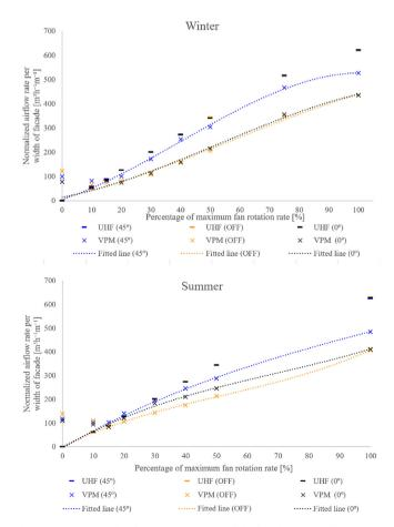
**Fig. 9.** The normalized airflow rates per width of the façade measured by the UFM and the VPM method. The figure shows the airflow rate profile obtained by fitting the measurements obtained by the UFM and the VPM method.
