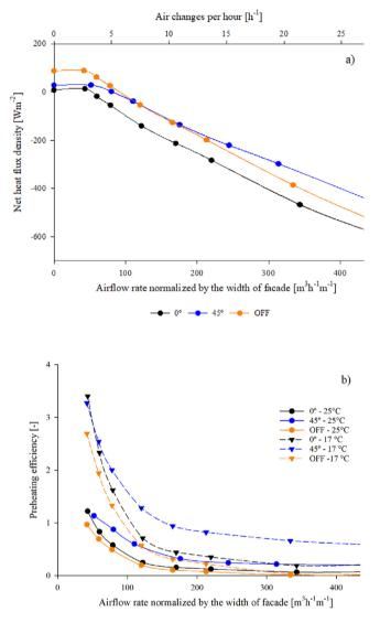
**Fig. 5.** The combined effect of mechanical ventilation rate and venetian blind set up on a) the net heat transfer and b) preheating efficiency (right) in the considered mid-season/winter conditions.
