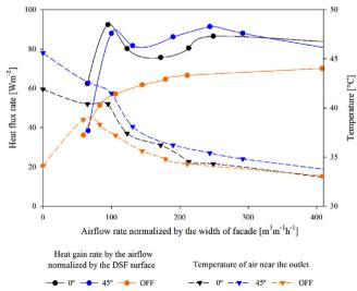
**Fig. 6.** The combined effect of mechanical ventilation rate and venetian blind setup on the normalized heat gain rate by the airflow and temperature of the airflow near an outlet in a) mid-season/winter and b) summer conditions.
