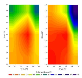
**Fig. 10.** Distribution of the relative deviation of the solar irradiance measured on the DSF surface in relation to the values measured in the central part for the summer (left) and winter period (right). The dimensions are scaled according to the width of the double glass façade (W).
