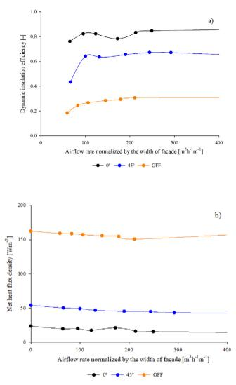
**Fig. 8.** The combined effect of mechanical ventilation rate and venetian blind set up on a) the dynamic insulation efficiency and b) net heat transfer (right) in the considered summer conditions.
