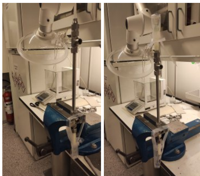
Figure 16: The procedure of sealing the module from both ends using epoxy glue
