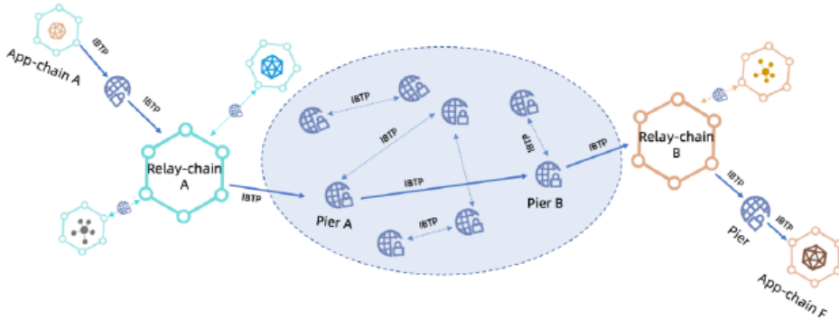
Figure 5: The BitxHub architecture, with different App-Chains (Blockchains), Relay-Chains for intercommunication, and Cross-chain gateways (in image called Peers) for setting up the IBTP between sender and reciever
