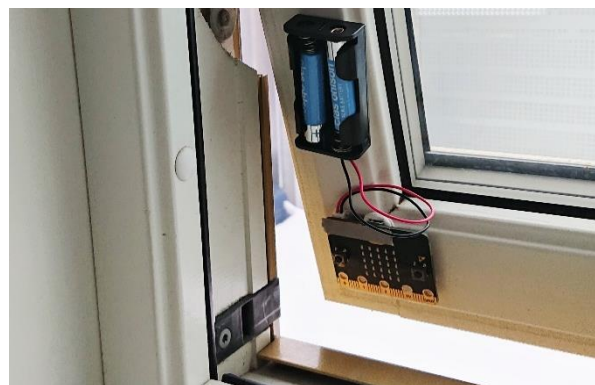
Figure 1. Sensor logging the window opening angle.
