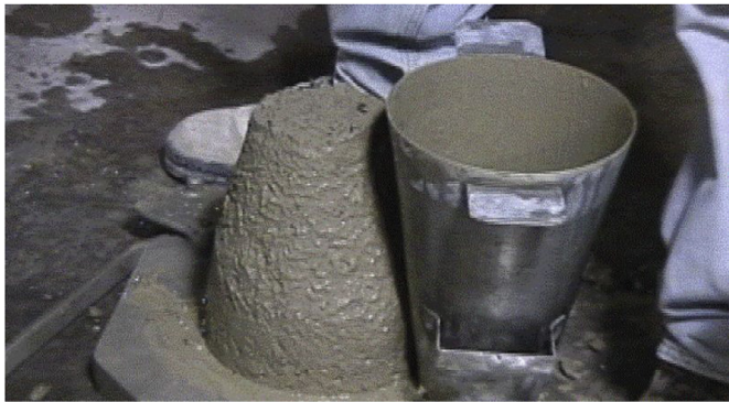
Fig. 5. Slump test of 20% SFA-based concrete as an example.
