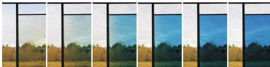
Figure 2.3. Six different coloration states of a complementary electrochromic device with electrochromic layers made with tungsten oxide and Prussian blue 74 .
