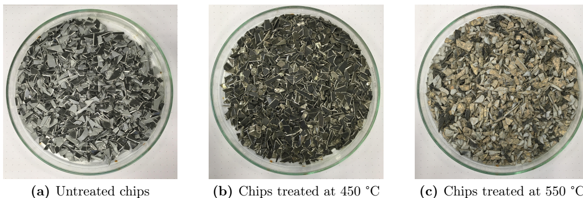
Figure 4.18: Colour changes of untreated chips and chips thermally treated at 450 and 550 °C
