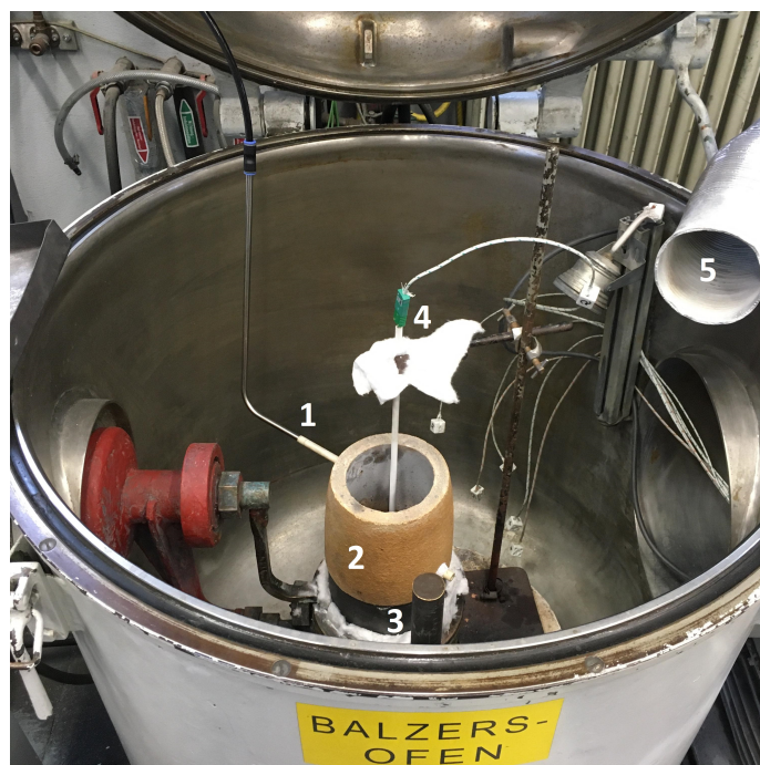
Figure 3.3: Furnace setup for remelting trials where; 1=Argon gas inlet, 2=Lid, 3=Crucible, 4=Thermocouple, and 5=Exhaust pipe
