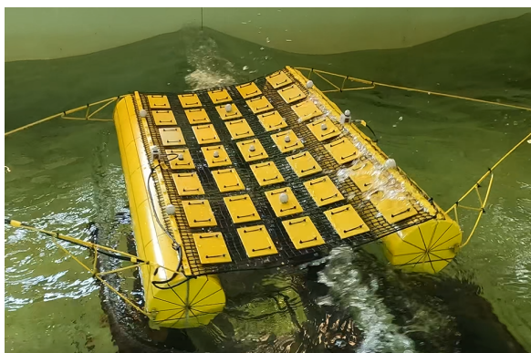
(a) Overtopping waves
