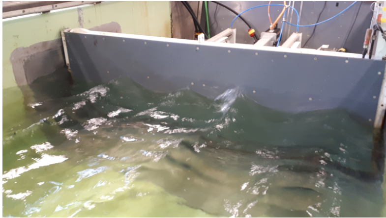
Figure 4.7: Transverse sloshing in the wave tank observed for wave periods T \leq 0.5 , amplified or triggered by changing the tension in the solar deck while the wave maker was running, introducing additional waves in the tank basin.
