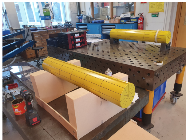
Figure A.2: Picture from the cylinder production. Painted yellow with black lines. A water line was also included at a later point in time. The small beam with screws along the cylinders can here be seen. The purpose of these was to fix the solar deck net to the cylinders.
