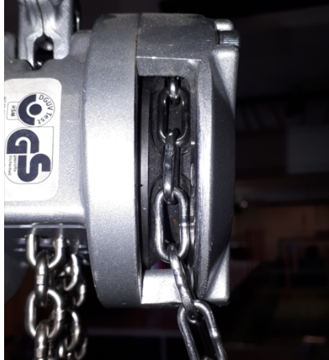
Figure 3.3: The locking mechanism of the chain hoist used in the model tests in this thesis.
