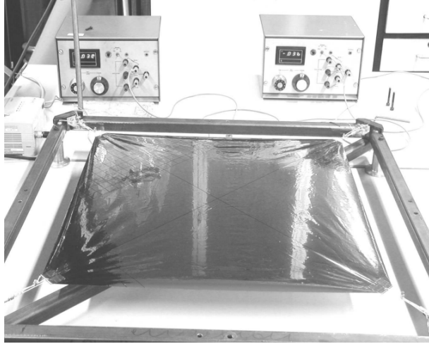
Figure 3.9: Wrinkles in a square membrane tensioned in the diagonal directions, where the diagonal forces are equal, or having a 1:1 ratio. Photo courtesy of Y. Wesley Wong and Sergio Pellegrino from Wong and Pellegrino 2006 .
