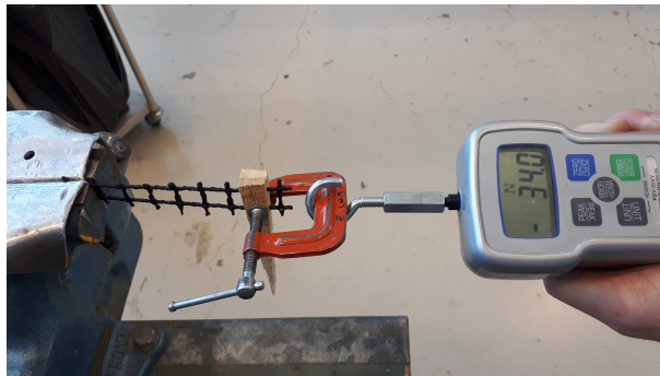
Figure A.4: Testing the ultimate strength of the net in the same direction that tension will be applied during model testing. Here the force measurement shows approximately 34 N.
