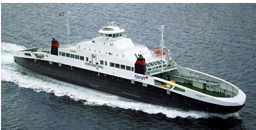
FIGURE 3. Example of double-ended ferry
