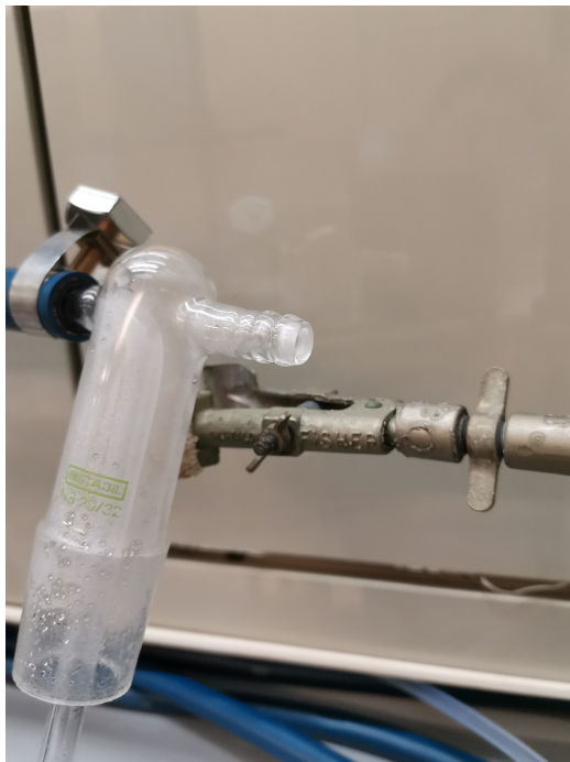
Figure 25: Formation of white coating on the outlet of the gas bubbler as seen in several of the experiments done.
