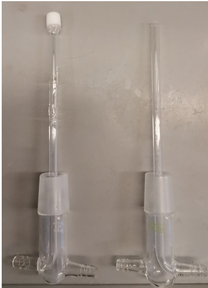
Figure 15: Comparison between porous bubbler "level 0" (left) and standard bubbler (right).
