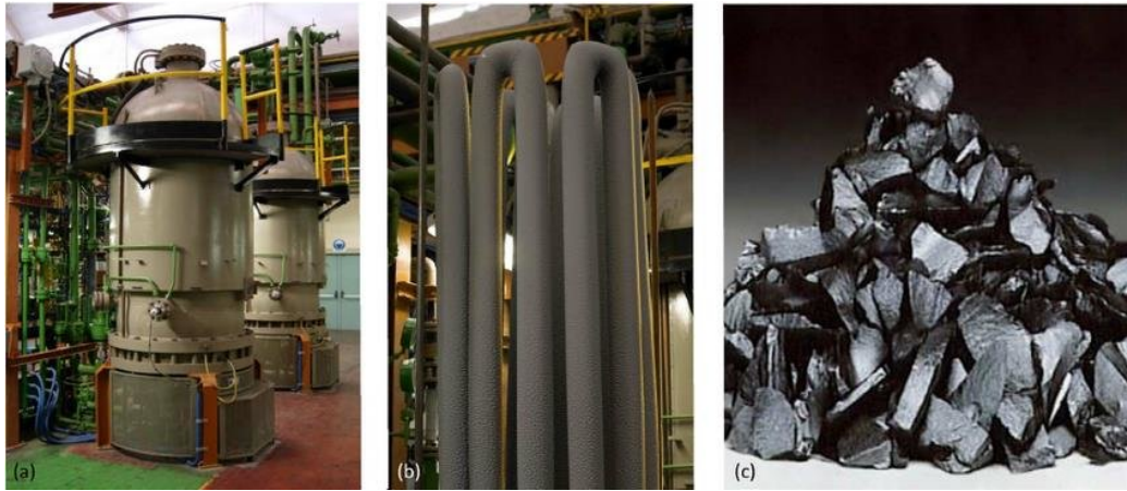
Figure 7: (a) Basic Siemens reactor. (b) As grown polysilicon rods after a reactor run. Current generation reactors have many more rods. (c) Final polysilicon chunks [5] .
