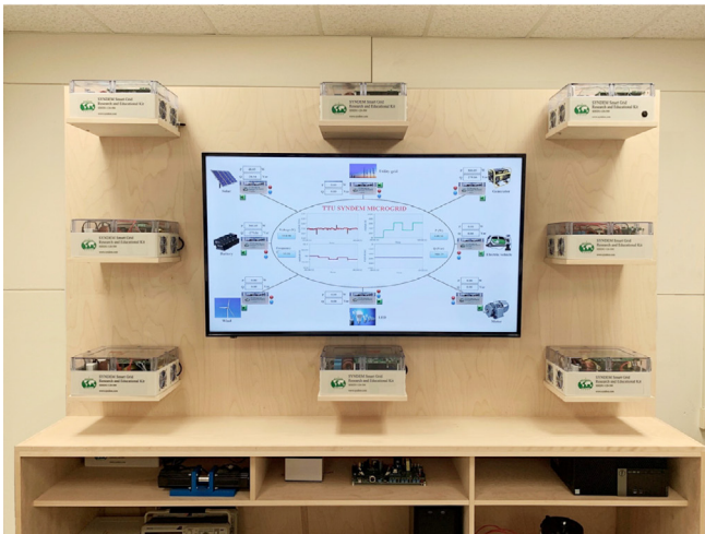
Fig. 12. Texas Tech SYNDEM Microgrid built up with eight SYNDEM Smart Grid Research and Educational Kits
