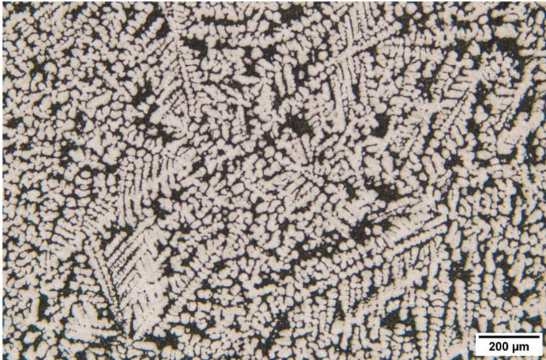
Figure 13. Enlarged light microscope (LM) image of a ground and polished cross-section of an inner part of the bead shown Figure 9. Dendrites of silver (white) are surrounded by solidified melt of lead and/or lead oxide, silver, and copper and/or copper oxide.
