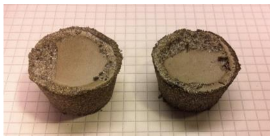
Figure 1. Replica bone-ash cupels. Dimensions of paper squares: 5 × 5 mm (Lohne et al., 2021, this volume).
