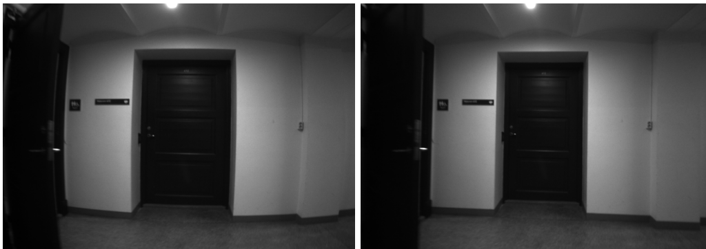
Figure 2: Comparing a raw, undistorted image (left) with the effect of applying the radial and tangential undistortion model (right).
