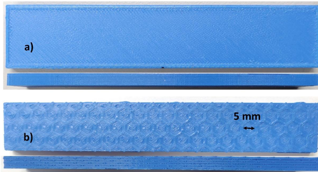
Figure 3.1: a) Specimen of Solid PLA specimen without having hexagonal structure b) Solid PLA specimen with hexagonal structure
