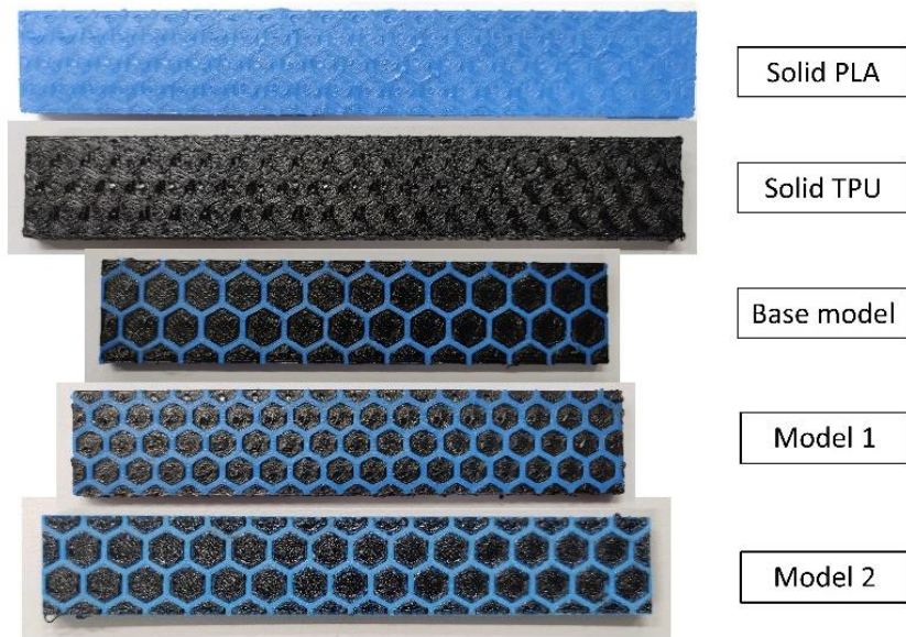
Figure 4.10: Reverse structured 3D printed specimens (Base model, Model 1, Model 2) where hexagonal platelets are made of TPU
