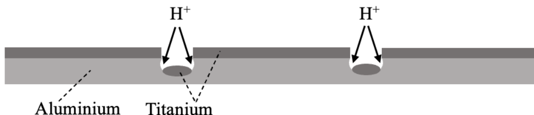
Figure 5.1: Simple sketch of the cross-section of an aluminium substrate containing pits, coated with titanium. Only partial coverage of titanium in the pits.
