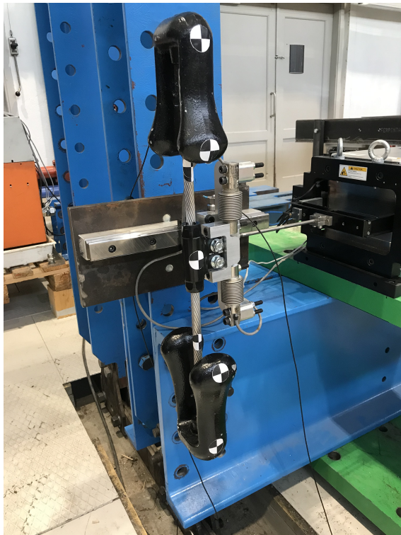
(a) Stickers on the damper.
