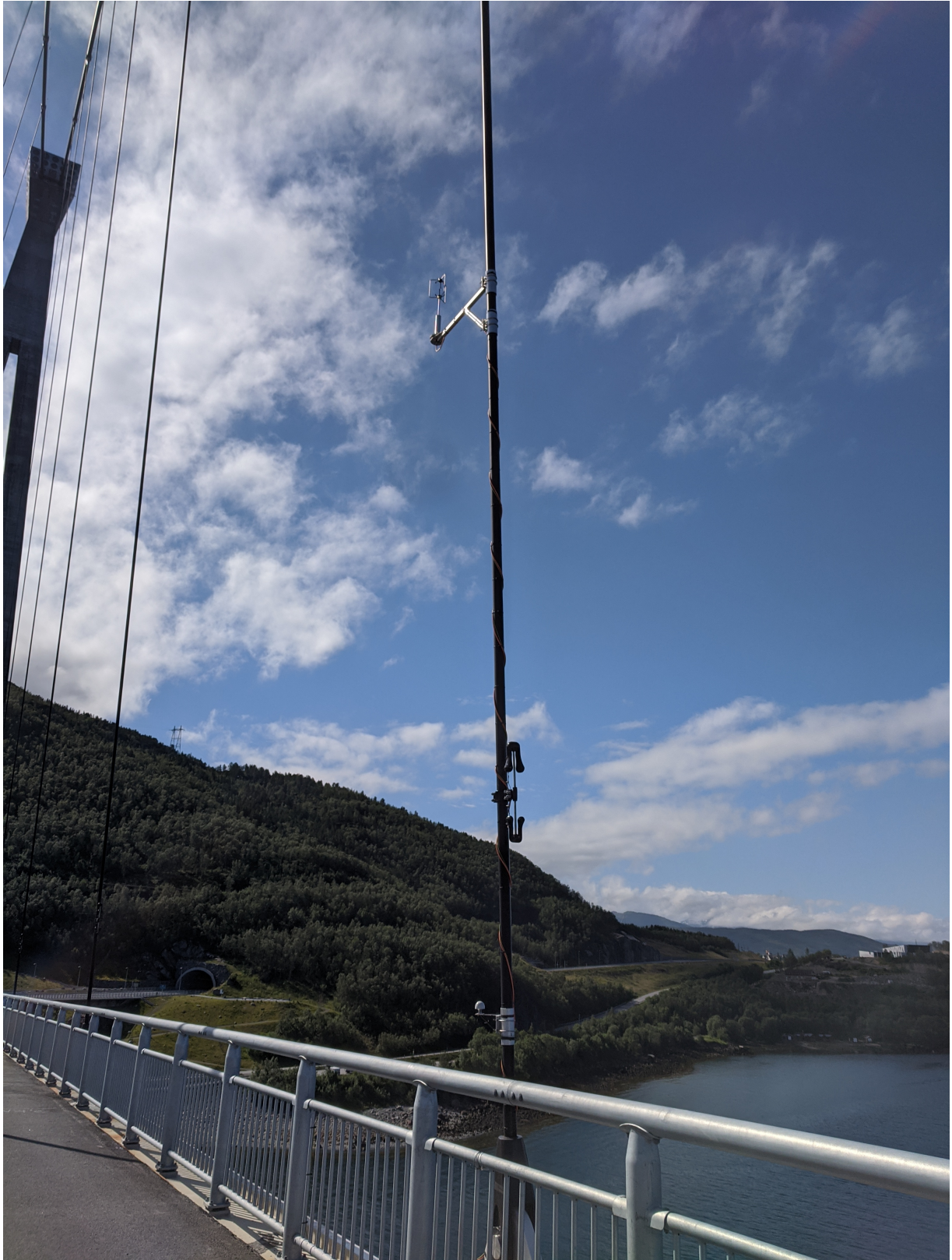
Figure A.2: Anemometer at hanger 7, mounted to the south-side of the hanger.
