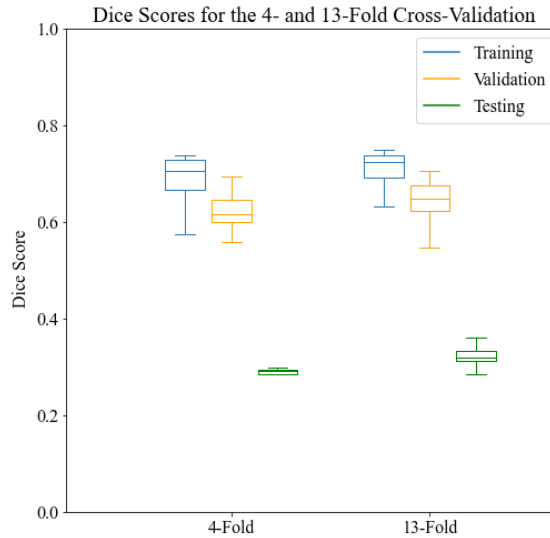
Figure 4.7: Box plot showing average values for the dice scores achieved from the training, validation and testing of the 2D U-Net model for both the 4-fold and 13-fold cross-validation.
