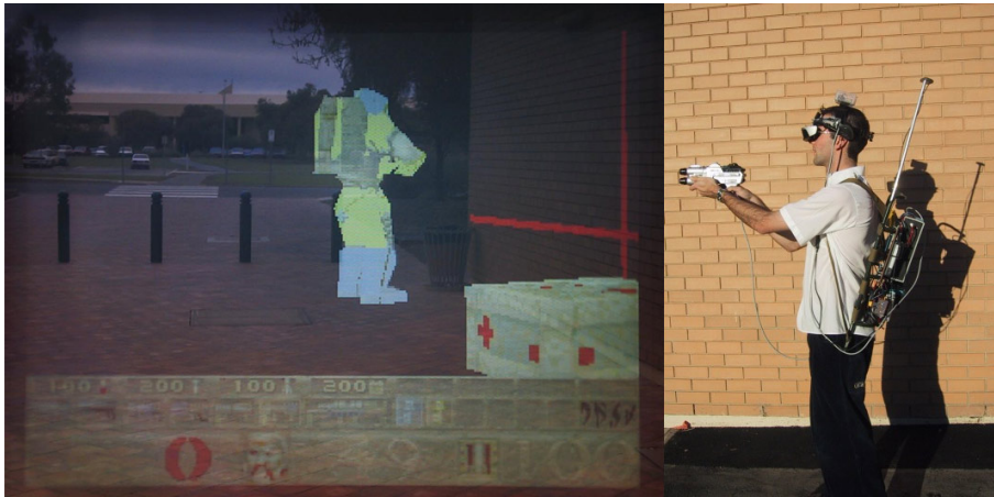
Figure 5: ARQuake setup. A player wears augmented reality goggles, and may then see the Quake UI integrated with the real world. [40]
