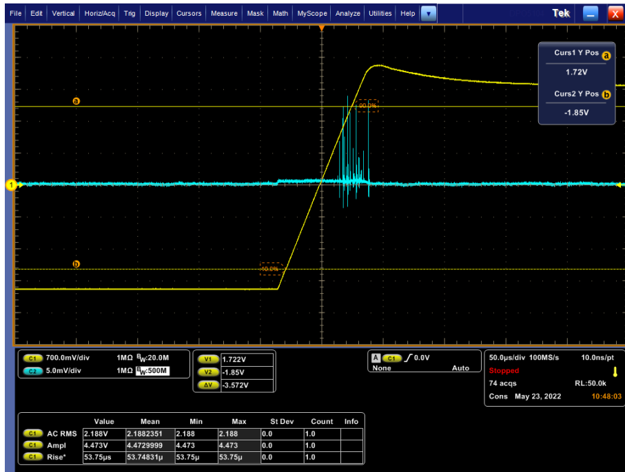
Figure B.2.5: Oscilloscope screenshot with 50 Hz square wave voltage, with a 300 pF parallel capacitor, showing the measurement of rise time
