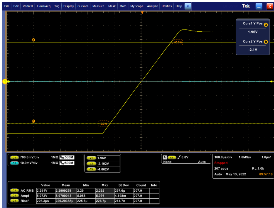
Figure B.2.4: Oscilloscope screenshot with 50 Hz square wave voltage, with a 1 nF parallel capacitor, showing the measurement of rise time
