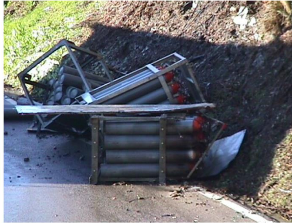
Figure 1.8: CGH 2 cylinders fallen onto the road (Pilo et al., 2005)
