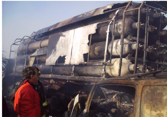
Figure 1.6: CGH 2 tube trailer after the accident (Pilo et al., 2005)
