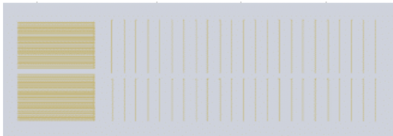
Figure 3.6: Layout of the laser surface remelting of the wedge cast tip
