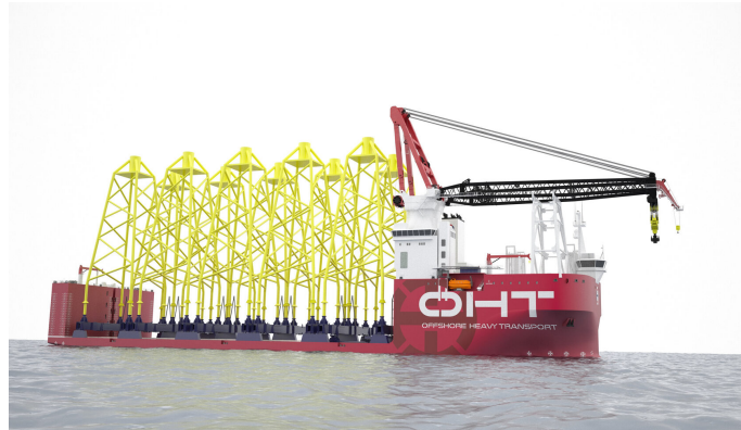
Figure 18: An illustration of the Seaway Alfa Lift carrying jackets.
