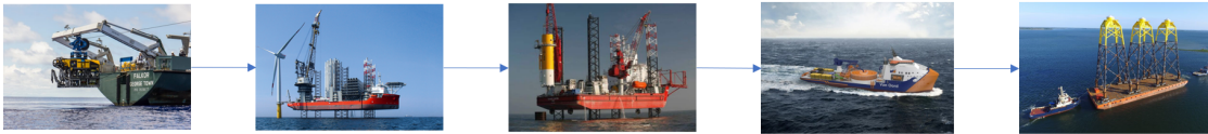
Figure 13: The system boundary: Use of ROV-vessels to prepare decom. operations, the disassembly of WTGs, the removal of foundations, recovery of cables, and transportation back to shore.
