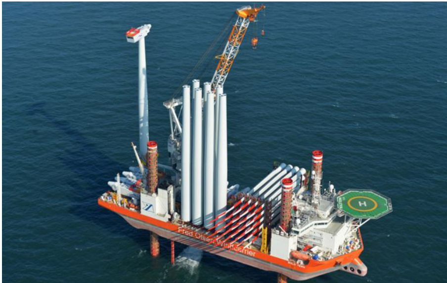
Figure 22: A typical jack up SPIV with turbines mounted vertically to the deck.
