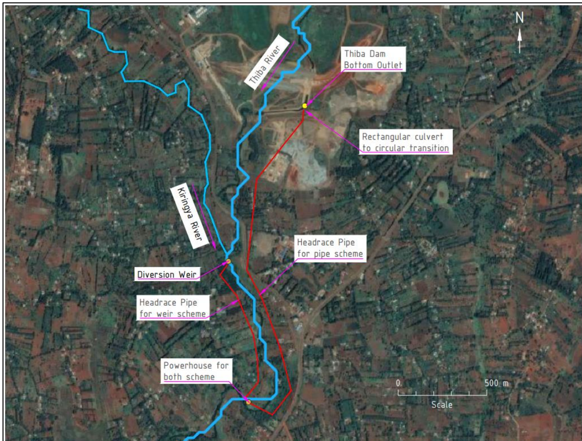
Figure 5-5: Proposed layout of two schemes for retrofitting of Thiba Dam. Scheme towards the right side of the river represents the layout of diversion weir scheme and left side of the river represents the layout of pipe scheme.
