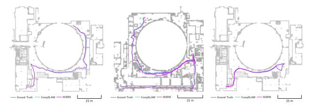
Figure 23: CompSLAM (blue) and M3RM (magenta) trajectories executed onboard the CERBERUS robots against ground truth (green). *Left:* ANYmal Badger, Urban Alpha 2 mission. *Middle:* ANYmal Bear, Urban Beta 2 mission. *Right:* Alpha Aerial Scout, Urban Alpha 2 mission.
