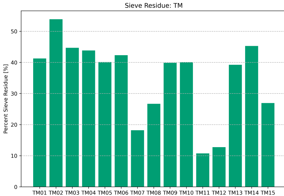
Figure 34: Sieve residues of the TM samples given in percent.
