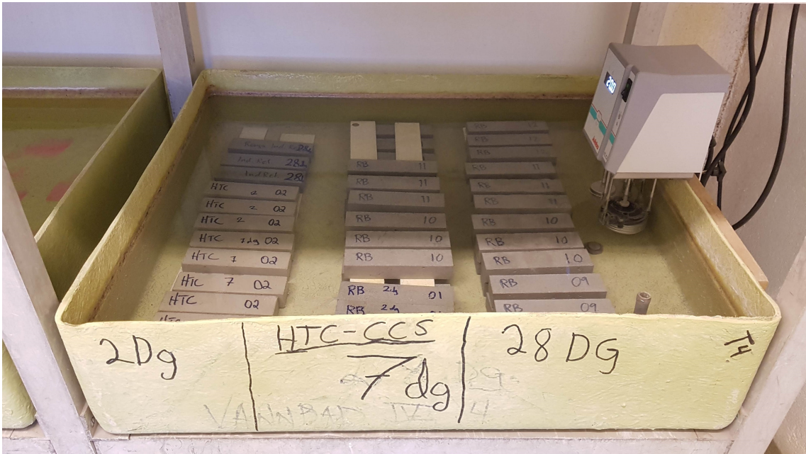
Figure 25: Mortar prisms stored in a water tank until strength tested.
