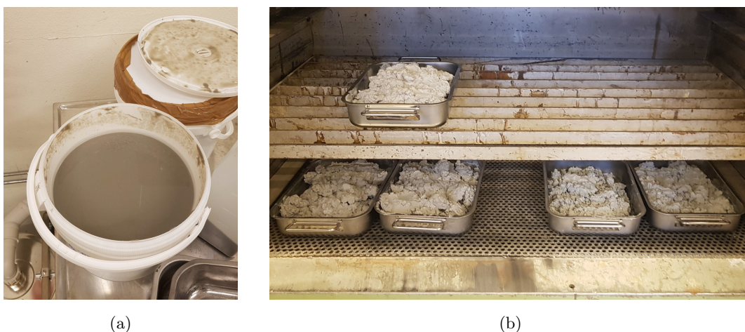
Figure 13: (a) washing sludge as it was received wet from the industry. (b) material to dry in the oven.
