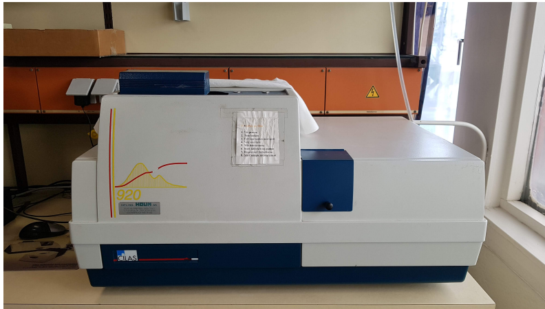
Figure 18: Cilas Particle Size 920 used for the particle size distribution analysis.
