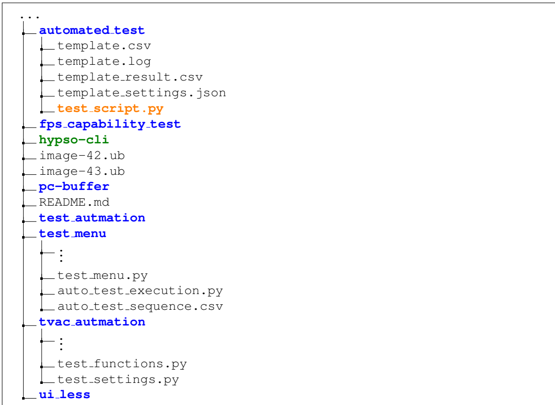
Figure 11: Structure of assembly-integration-test repository. Hypso-cli in green is the executable created by building the code in hypso-sw repository 2.4.1, while test_script.py is the main test script for the test framework created in this thesis.
