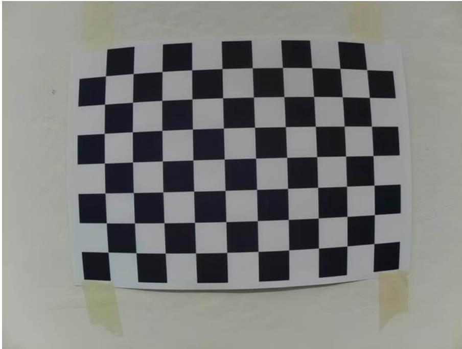
Figure 3.10: Distorted picture from the camera
