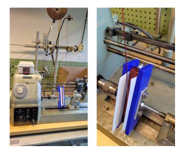
Fig. 17. Winding process of the coils
