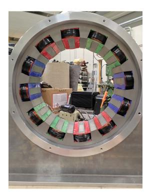
Fig. 19. All coils glued in the stator
