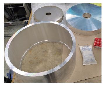
Fig. 14. Stator housing and cover
