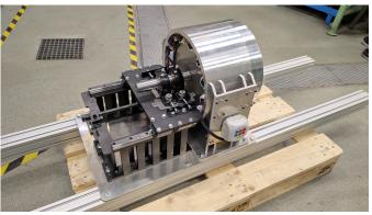
Fig. 24. First attempt at aligning the 22-pole rotor
