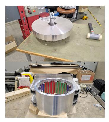
Fig. 21. Entering the first rotor
