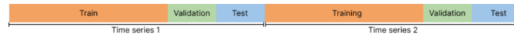
Figure 6.2: Illustration of how multiple time series are concatenated for the global method
