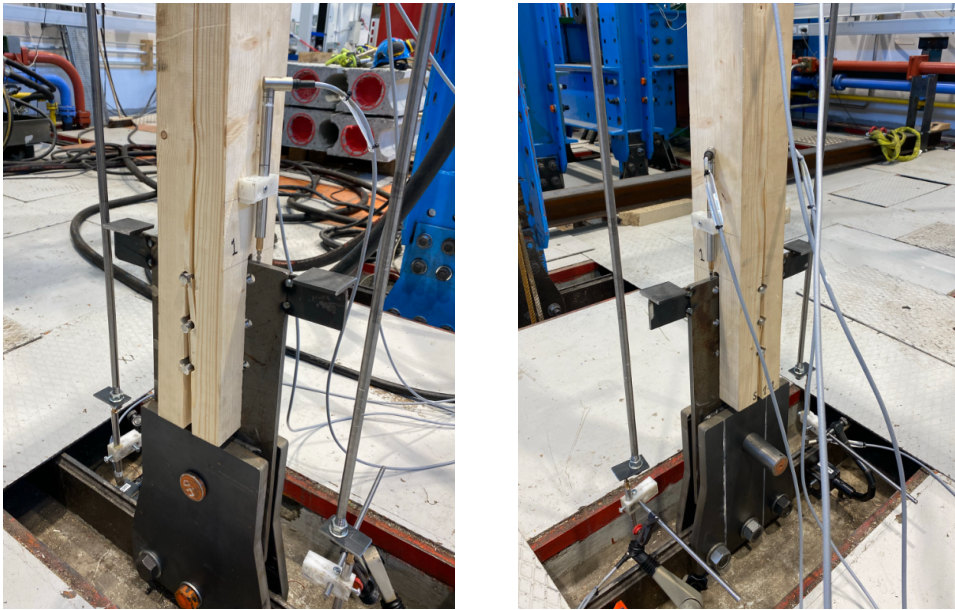
(a) Failure of S1-1, side 1
