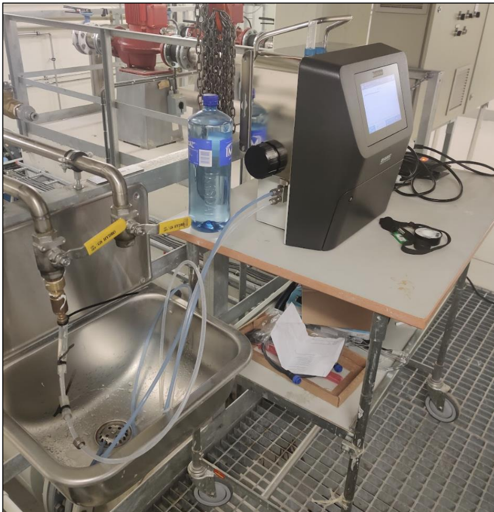
Figure 17. Set up of BactoSense FCM at VIVA. The inflow to BactoSense was connected to the faucet using adapters. The flow in and out of the BactoSense was constant.
