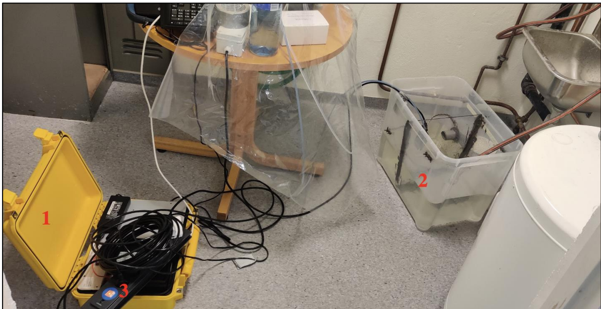
Figure 18. Set up for tracer study at Jakobsli pumping station. 1. Protection case that contains data logger. 2. 70L plastic box where the measurement of conductivity takes place. 3. Extension cord for power supply.
