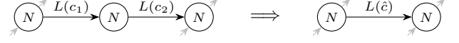
Fig. 2: The second operation, illustrated for n = 2 , merges sequential links and nodes into a single link. The grey arrows indicate potential connections which are not relevant to the operation.
