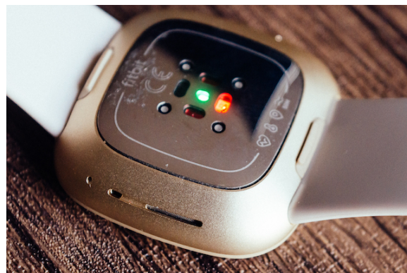
Figure 7. Fitbit HR sensor showing multi-path optical heart rate sensor.
