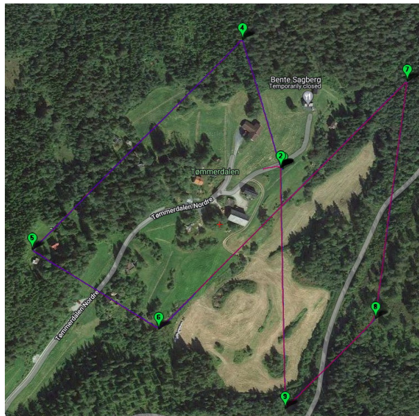
Figure 4.30: Flight plan for all 3 flights on 30.05. Flight 2 is visualized here.
