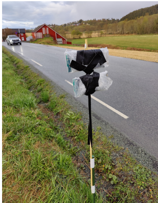
Figure 4.7: Pole consisting of a metal and wooden part, with two nRF52833 Development Kits attached on top.
