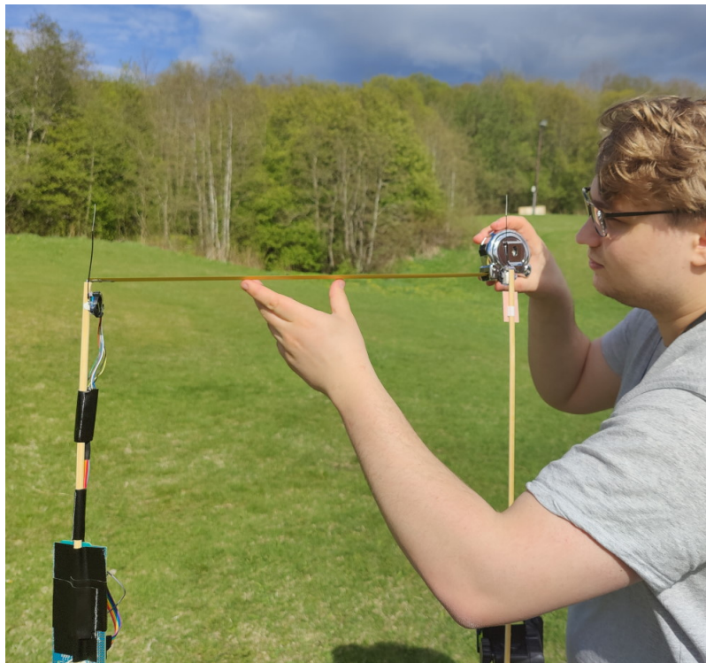
Figure 4.4: Experimental setup for orientation test 2. Two monopole antennas and the distance between them measured with a tape measured.
