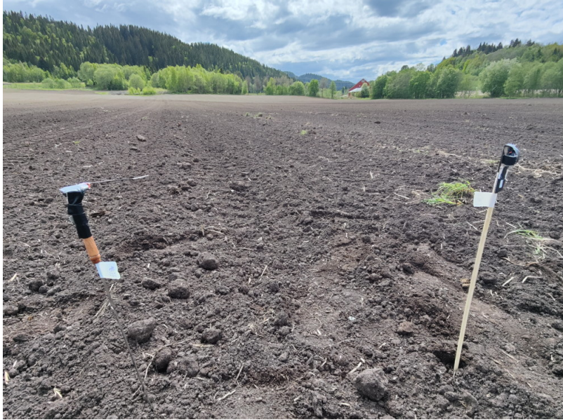
Figure 4.17: nRF528xx chips (one with integrated PCB antenna, one with Monopole) rotated the same way, with antennas oriented horizontally.
