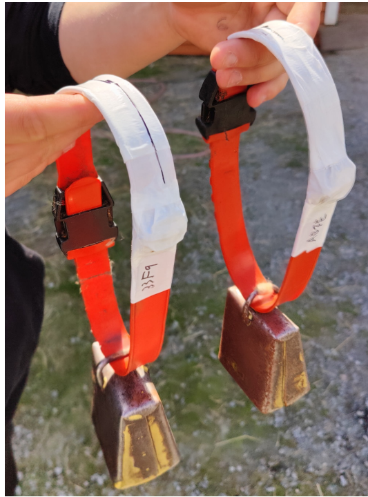
Figure 3.4: First version of our prototype tag, mounted to sheep collars. The black line shows where the antenna is, and the thicker black line where the antenna's radiating element is.
