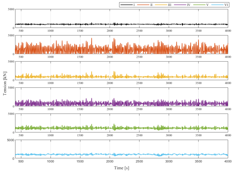
Figure B.1: Time series of mooring line tension in mooring line 3 during DLC 6.1 acting towards 180^\circ for all systems.
