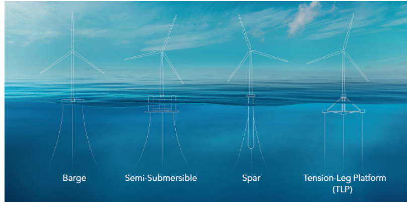
Figure 2.1: Main concepts for offshore floating wind [8].
