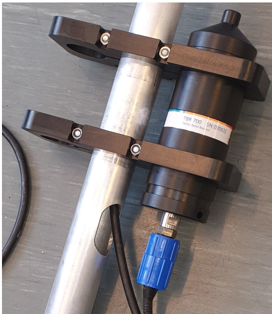
(a) TBR bracket and lower cable entrance hole, taken by the author of this thesis.
