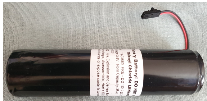
Figure 3.6: Double D cell thionyl chloride lithium battery. Picture taken by the author of this thesis.
