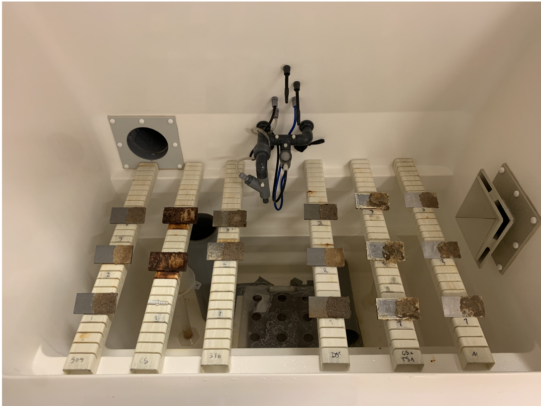
Figure 5: Picture of the samples after 334 hours of exposure in the salt-spray chamber.
