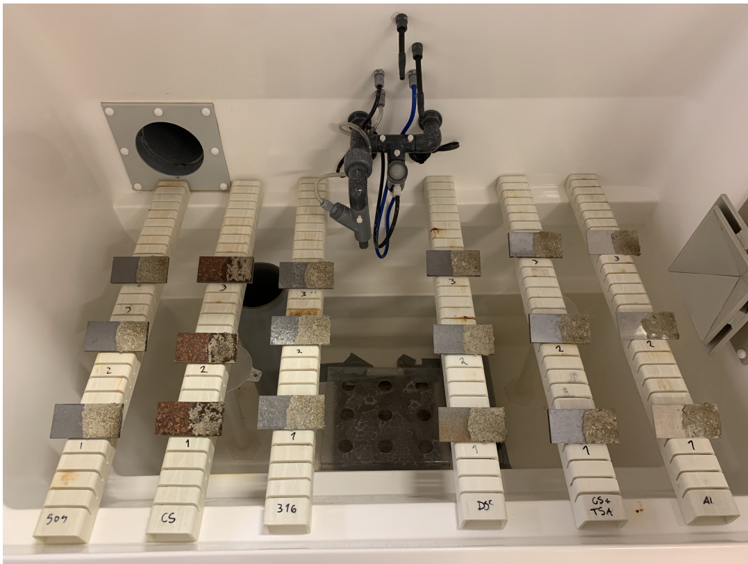
Figure 4: Picture of the samples after 49 hours of exposure in the salt-spray chamber.
