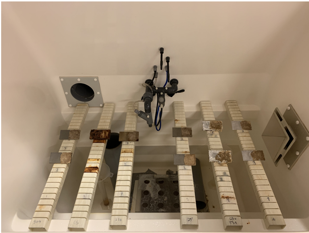
Figure 6: Picture of the samples after 592 hours of exposure in the salt-spray chamber.
