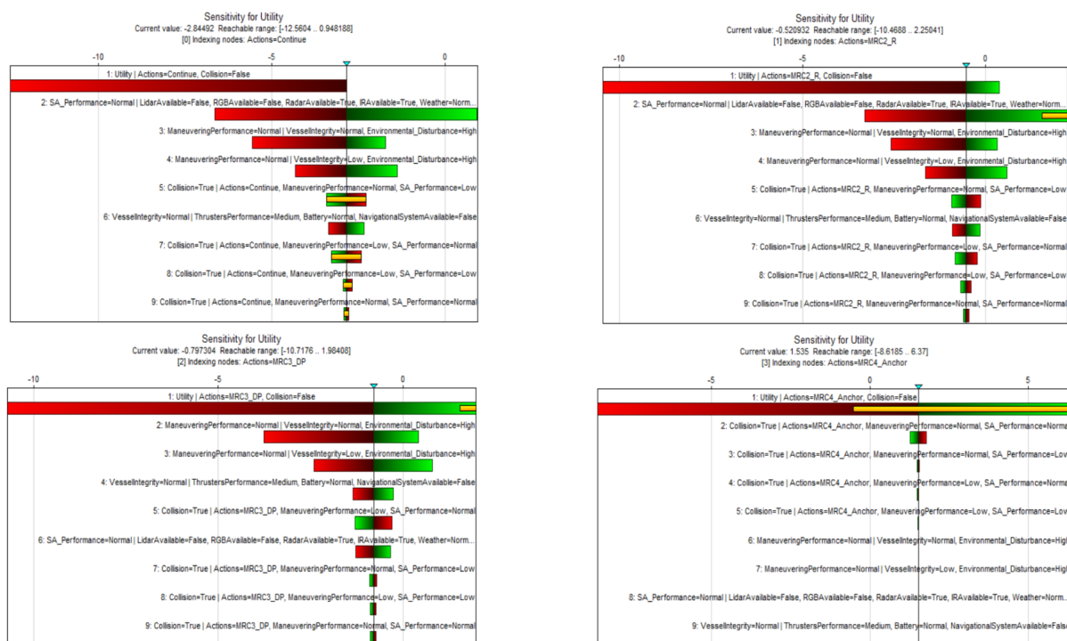
Figure 3.3: Third sensitivity tornado of Model 1 with Lidars failure, RGB failure, low lighting, Navigational system failure, Thruster Performance, high Wind Speed and high Current Speed . From top left is Continue, MRC 2, MRC 3 and MRC 4.
