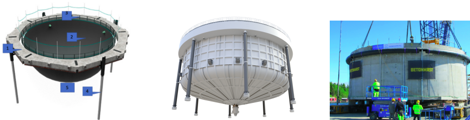
Figure 1.1: AkvaFuture's flexible system(illustration: Akvadesign), Aquafarm's semi-rigid structure Neptune(illustration: Aquafarm) and Dr.tech Olav Olav Olsens rigid cage Salmon Home nr 1(illustration: Olsen (2020)).
